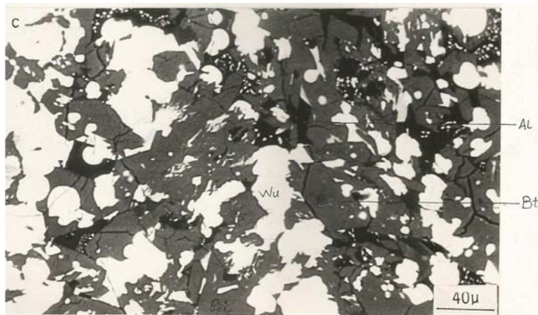
Figure 11. (40μ). Shows intergrowth texture exhibited by DSC slag minerals (belites and wustites, prominently).
