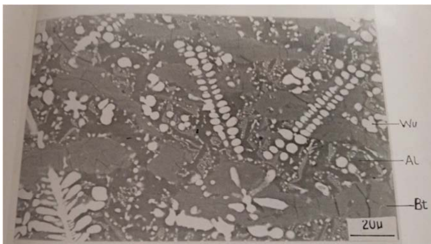
Figure 7. Shows dendritic wustite (Wu-white) in contact with lenticular belite (Bt- light to dark gray) and dark aluminate (Al) of no definite shape. Some wustite grains occur on aluminates.
