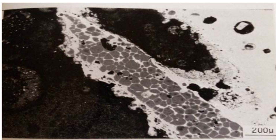
Figure 2. Shows round, rectangular and angular (gray) periclase (MgO) crystals on both a mixed and wustite groundmass but always surrounded by a thin shell of wustite. The wustite had protected the periclase from possible inter-phase or liquid reactions.
