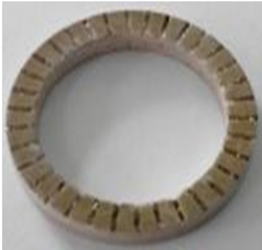
Fig. 6. Preparation of composite ring array.
