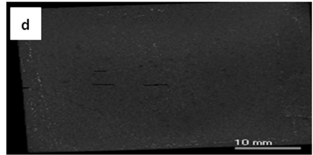
Figure 5. (a) SEM image of Cu/W85Cu/Cu; (b) The Magnified morphology of Cu/W85Cu/Cu composites; (c) Microstructure and line analysis of chemical composition at Cu/W85Cu/Cu interface (Blue curve represents Cu, light green curve represents Ni and red curve represents Ag); (d) SAM image of Cu/W85Cu/Cu solder joints.
