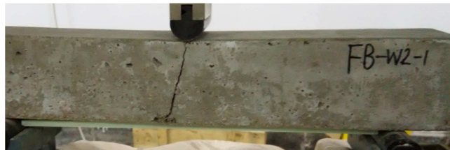
(c) failure pattern of FB-W2 concrete specimen
