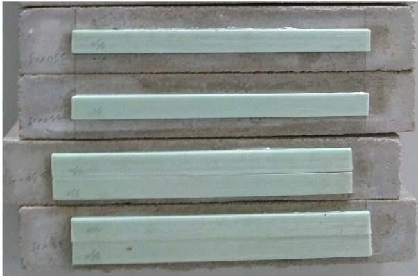
Fig. 2. FRP reinforced concrete specimen.
