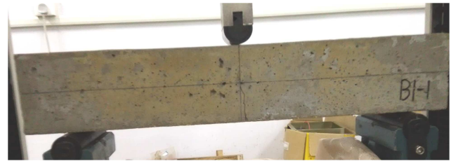
(a) failure pattern of plain concrete beam
