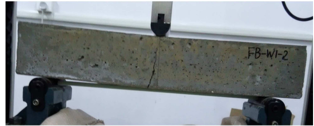
(b) failure pattern of FB-W1 concrete specimen
