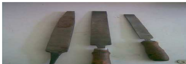
Fig. 8. Abrasive file used for wear test (left to right rough (double cut), medium (double cut) and soft (single cut)).
