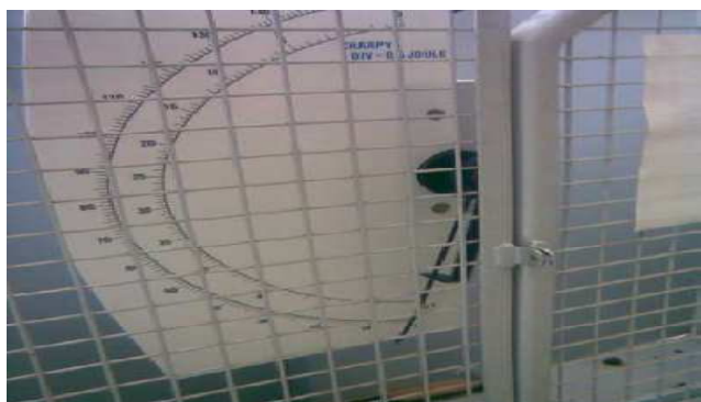
Fig. 7. Charpy impact tester for toughness testing (T50).
