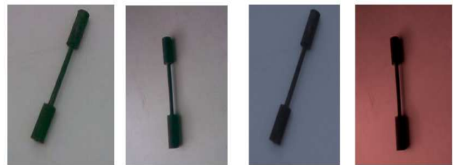
Fig. 3. Steel Specimen for tensile strength test.
