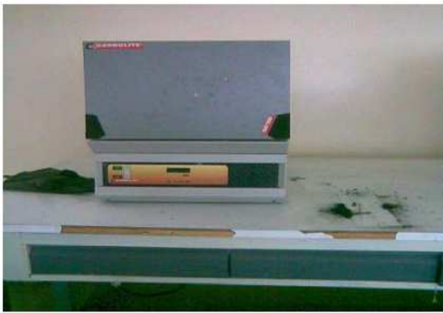
Fig. 5. Electrical furnace for carburization of steel samples.
