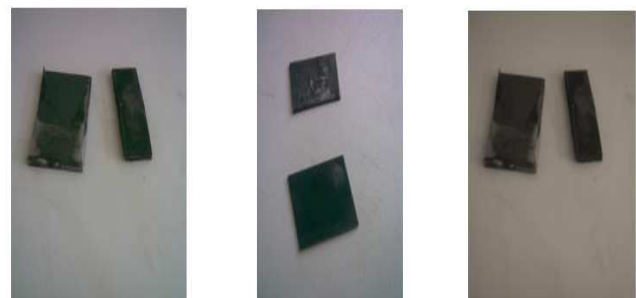
Fig. 4. Abrasive wear test specimens (Steel).
