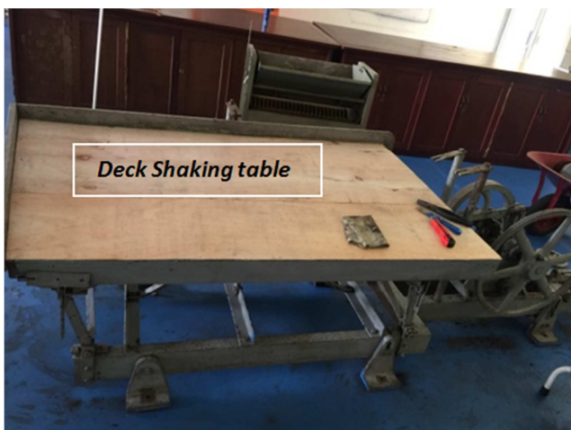
Figure 3. Results of Deck Shaking Table Design.
