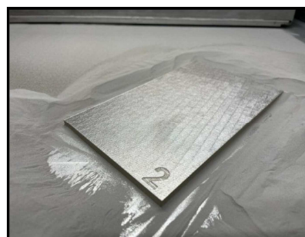
Figure 1. Additively manufactured plate of size 160x100x6 mm 3 .
