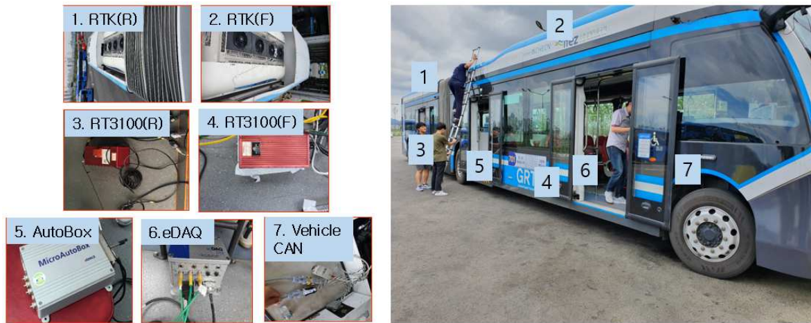
Figure 1. Test devices for the preparation of vehicle tests and the locations.
