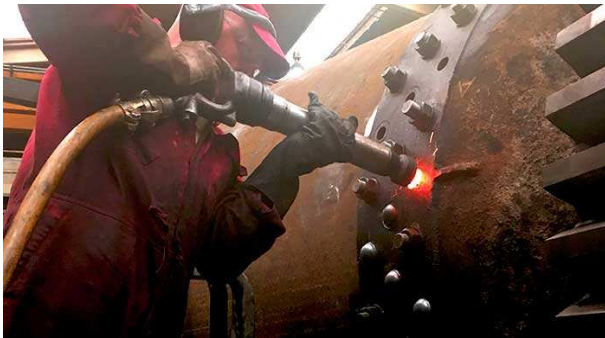
Figure 8. Hot rivet forge welding.
