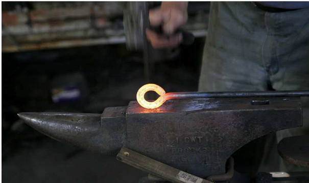
Figure 9. Blacksmith forge welding.
