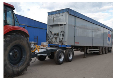
Figure 5. NPS 3250 grain truck semi-trailer with PSP-20 saddle trailer for work with a tractor in the field.
