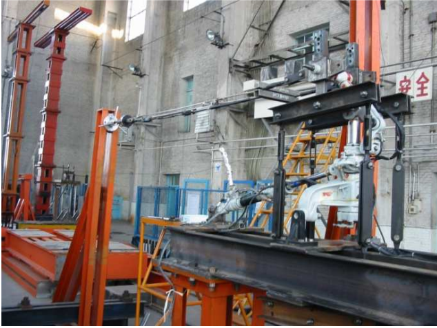
Figure 5. Load calibration of the front landing gear.
