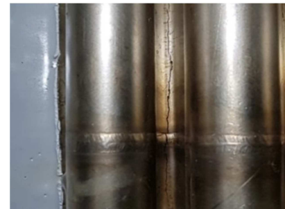
(b) Crack on surface of bellows part
