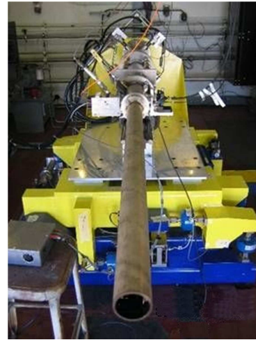
Figure 1. Detonation Tube.
