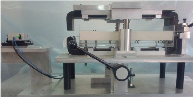
Figure 1. Magnetostrictive measurement device.
