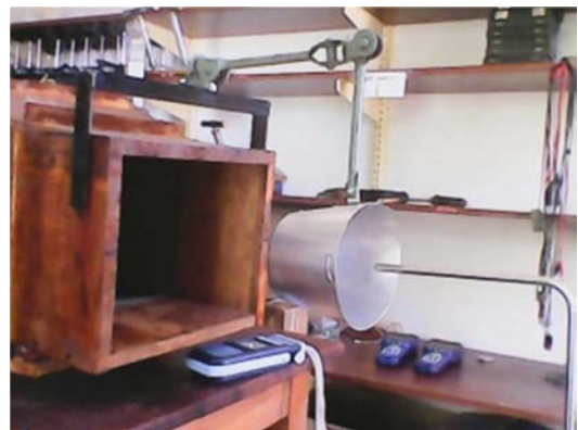
Figure 3. Experimental setup for the wind speed augmentation measurement.
