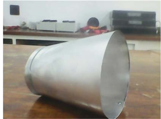
Figure 2. Conical diffuser of L/D=2 .
