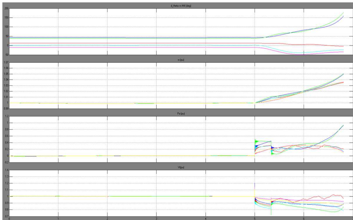
Figure 10. Transient in the 6-machine power system model, K_{Dv} = 3.3 , N = 180 is inputted to the SM G3-G6 in the areas 2, 3.
