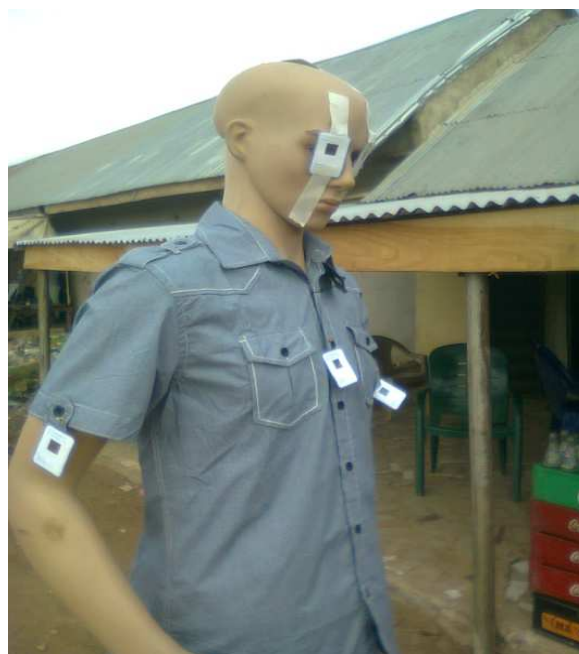
Figure 2. Dosimeters placed on plastic human figure to measure UV radiation
