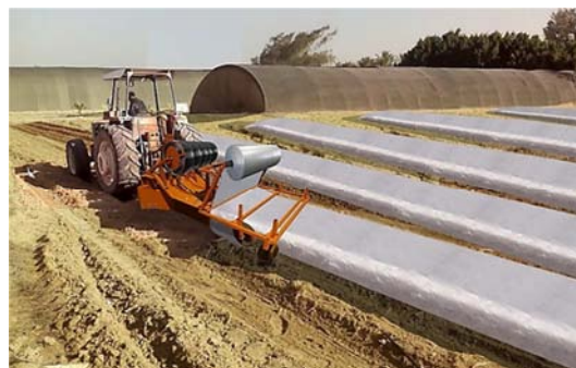
Figure 3. Developed mulching machine during the field experimental work.
