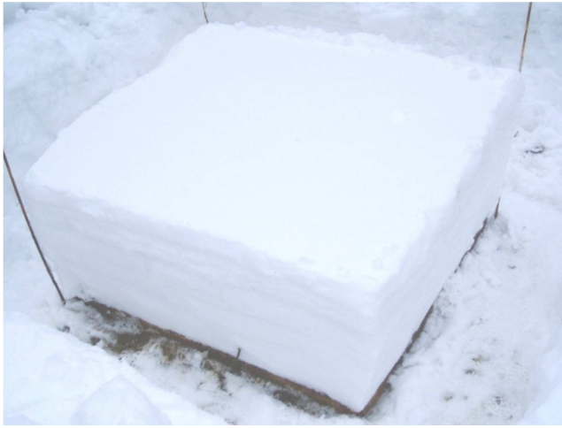
Figure 2. The lysimeter collector; of dimensions 1 m × 1 m.
