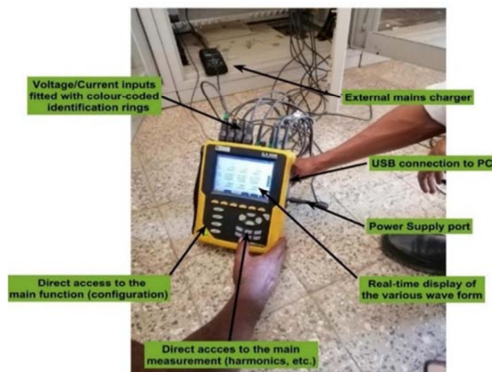
Figure 9. Chauvin Arnoux CA 8335 Power Quality Analyzer Installation.
