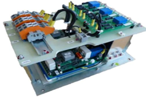
Figure 6. Auxiliary power supply system for railway system [21].
