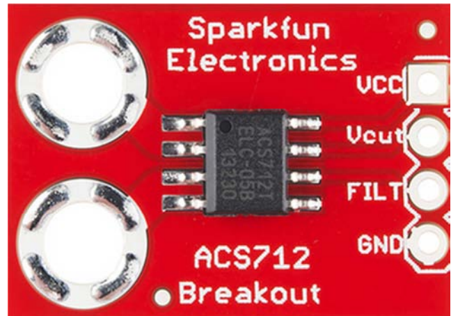
Figure 3. Current sensor (ACS712).
