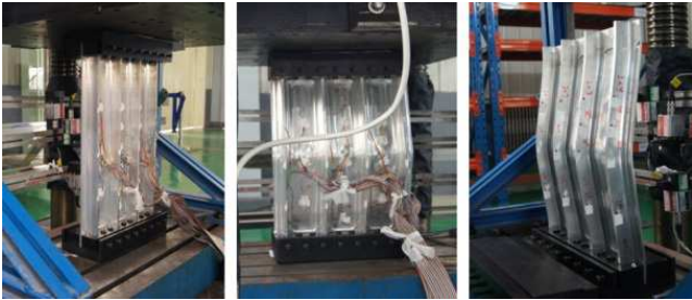
Figure 10. Before and after failure of “T” shaped integral panel during axial compression test.
