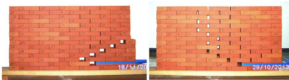
Figure 1. Two different yield lines for a same horizontal load location.
