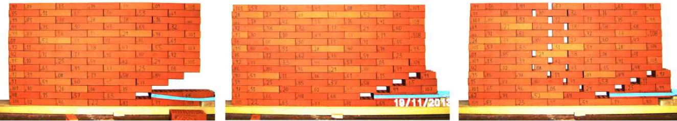
Figure 6. a- Post-collapse equilibrium, b- Mechanism of minimum, c- Mechanism near maximum.
