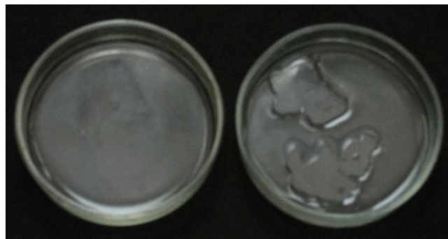
Figure 3. Left: 5 ml of water with an electric potential of -200 \text{ mV} cover all the bottom of a Petri dish. Right: 5 ml of water with an electric potential of +200 \text{ mV} do not cover the bottom of a Petri dish; the surface of such water decreases rapidly after mixing [3].
