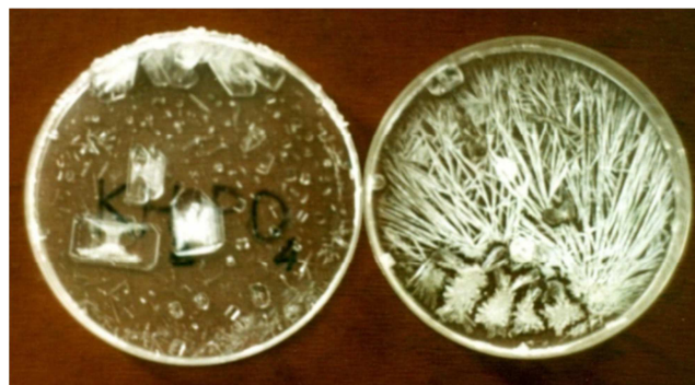
Figure 1. These are crystals formed in dried \text{KH}_2\text{PO}_4 solutions prepared with positively (left) and negatively (right) charged waters. The high surface tension of positively charged water forms compact crystals, both small and large (left), while the low surface tension of negatively charged water creates conditions for the formation of extended crystals (right) [1].
