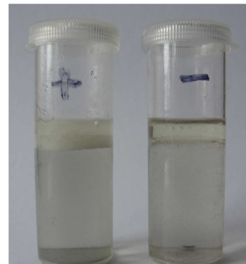
Figure 6. Suspensions formed by intensive mixing of oils with positively charged water do not stratify for hours and, accordingly, retain their milky white or yellowish color (left), unlike suspensions formed by intensive mixing of the same oils with negatively charged water, which stratify within minutes (right).
