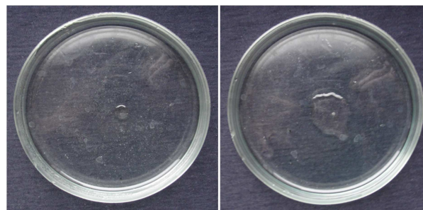
Figure 8. Left: a small oil drop on the surface of water with a potential of -500 mV looks like this. Right: a large oil spot on the surface of water with a potential of -500 mV looks like this; the shape of this spot remains unchanged due to the lack of interaction between the oil and the sufficiently negatively charged water.
