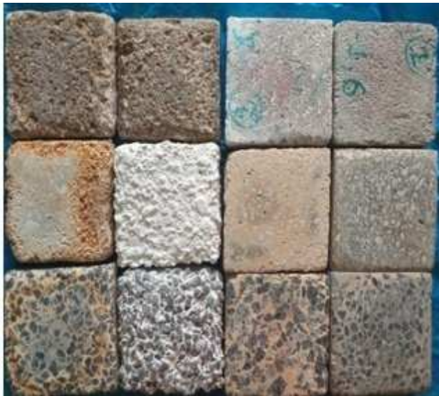
Figure 9. Surface condition of the samples after 35 days of immersion in HCl , H_2SO_4 , CH_3COOH and NaOH and (from left to right).
