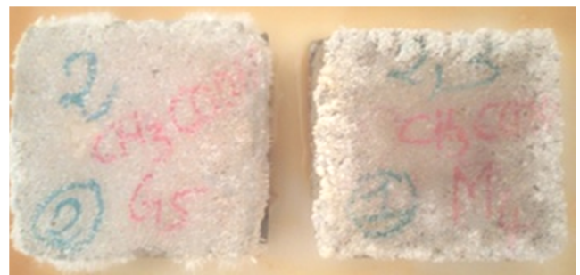
Figure 10. Surface appearance of specimens immersed in CH_3COOH .
