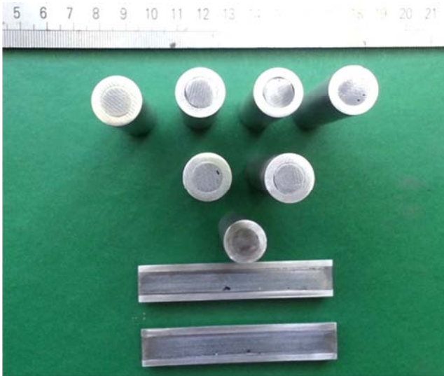
Figure 2. Bimetallic work-piece Al-Pb sleeve-core configuration.
