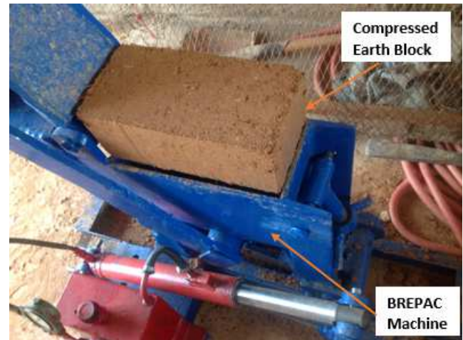
Figure 1. Moulding of Block with BREPAC Machine.
