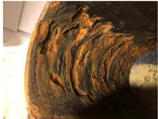
Figure 22. Bands of Fatigue Due to Water Hammer Pressure Waves.
