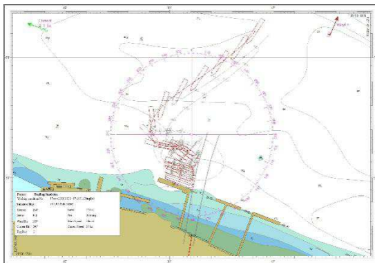
(a) Fully loaded, crosswind (onshore wind BF scale 6) turn for berthing
