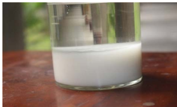
Figure 7. Nano-cellulose from okra fiber.
