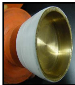
Figure 4. Hollow cathode electrode of 4cm diameter and 2cm depth
