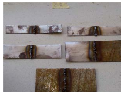
0.8 mm Welded Mild Steel Plate Specimen
