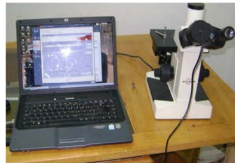
Figure 3. Accuscope Microscope with Camera (Serial no 0524011, Maker (Princeton, US)).
