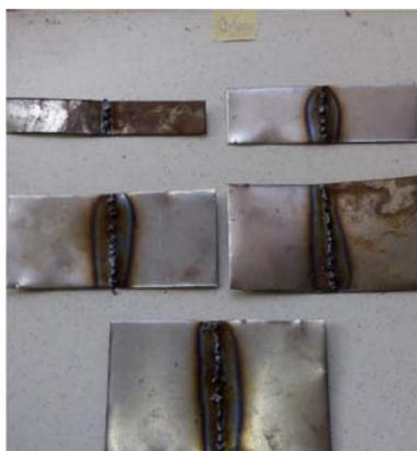
0.6 mm Welded Mild Steel Plate Specimen
