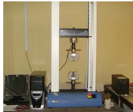
Figure 1. Universal Instron Machine, Model 3369, Maker (Instron).
