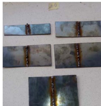
1.0 mm Welded Mild Steel Plate Specimen
