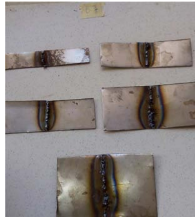
0.7 mm Welded Mild Steel Plate Specimen
