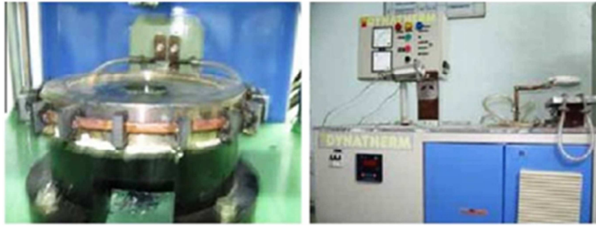
Figure 2. Induction Furnace Developed to draw the materials at elevated temperatures.
