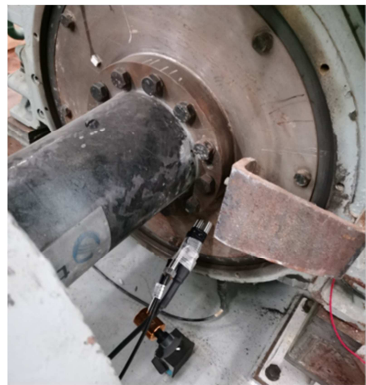
Figure 9. Speed Sensor and Inductive Magnet Piece.
