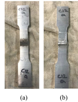
Figure 10. Sample for the UTS measurement (a) Weld surface (b) Root weld (penetration).
