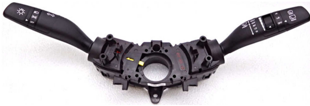
Figure 25. Steering column switches [24].
