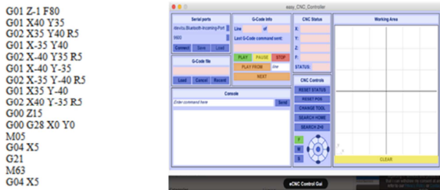
Figure 21. G-code and CNC control software GUI. [20].
