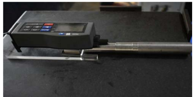
Figure 3. Surface roughness measurement.
