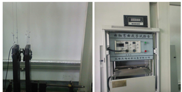
Figure 22. The Crank Throw Bend Fatigue Testing Bench.
