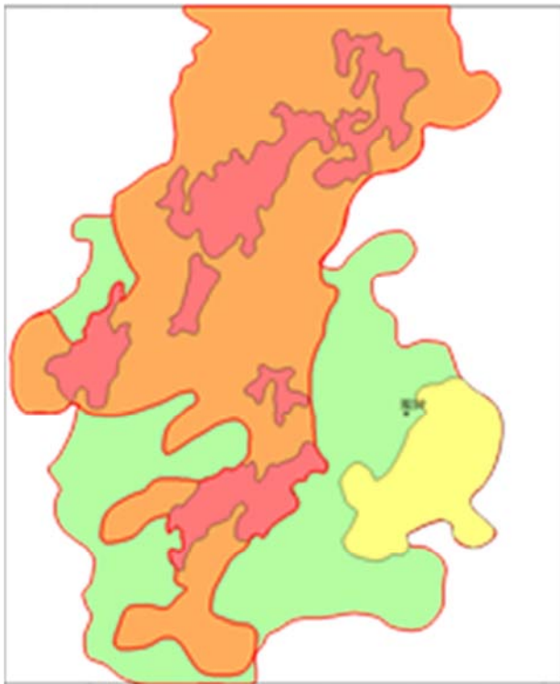
Figure 3. Distribution Diagram of Primary and Secondary Lithofacies of Volcanics in First Section of Yingcheng Formation.
