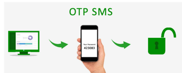
Figure 4. SMS OTP Principle: The OTP is generated by the service provider and sent to the mobile network operator (MNO) that delivers the OTP via SMS to the user.
