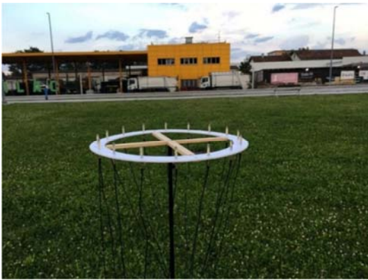
Figure 5. A uniform circular array with 16 G.R.A.S. Type 40PH omnidirectional microphones.
