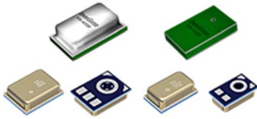
Figure 1. Different types of MEMS microphones [4].
