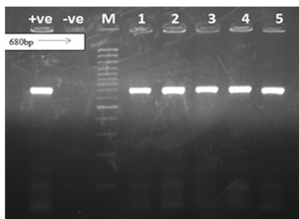
Fig. 3. Conventional PCR agarose gel picture of HBV positive samples mixed with ash of incinerated infectious waste, +ve control, -ve control, M (100bp marker), 1-5 samples.
