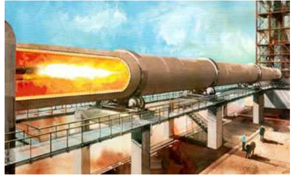
Figure 1. Typical rotary kiln showing the flame propagation and bed temperature
