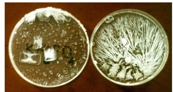
Figure 10. It is the crystals that formed after the drying of solutions of KH_2PO_4 prepared on water potentials of +250 mV (left) and -250 mV (right) [14, 15].
