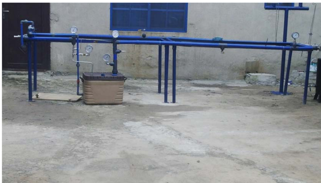
Figure 10. Frame Work of Laboratory Loop during construction.
