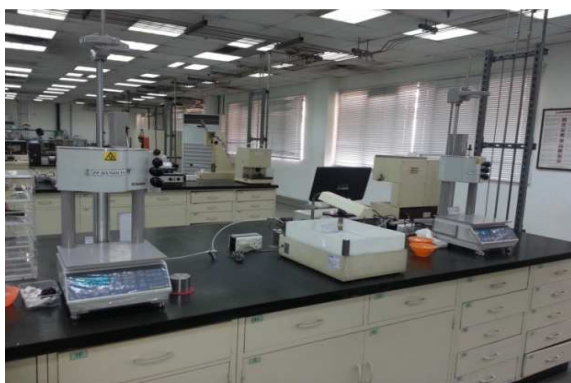
Figure 3b. Extrusion plastometer for MFI analysis.
