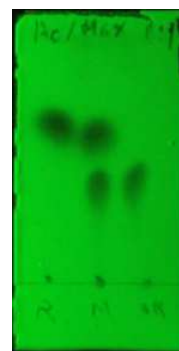
Figure 13. TLC of the reaction medium after 2 hours of reaction.
