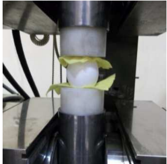
Figure 6. Placement of the sample inside the machine
