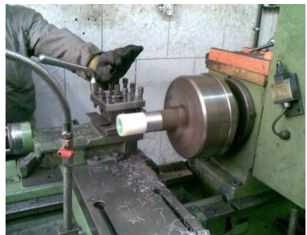
Figure 4. Turning for creating a seating base
